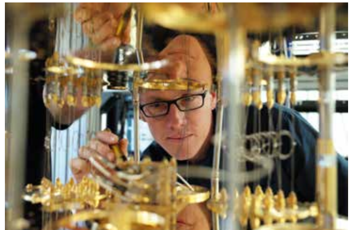
Stefan Filipp inspecting components of the cryogenic refrigerator used for quantum experiments.
