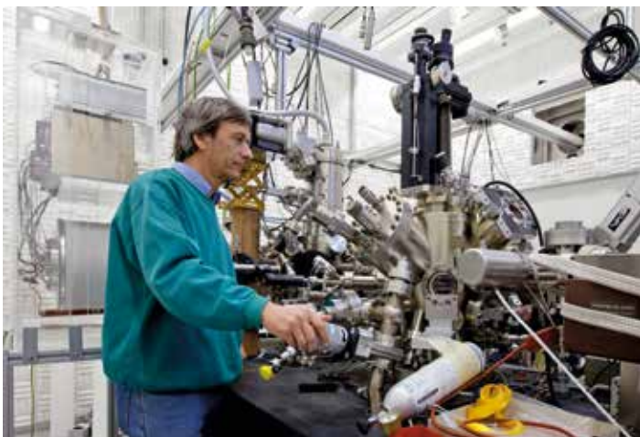
Rolf Allenspach with the spin-polarized scanning electron microscope (spin-SEM) in one of the noise-free labs.
