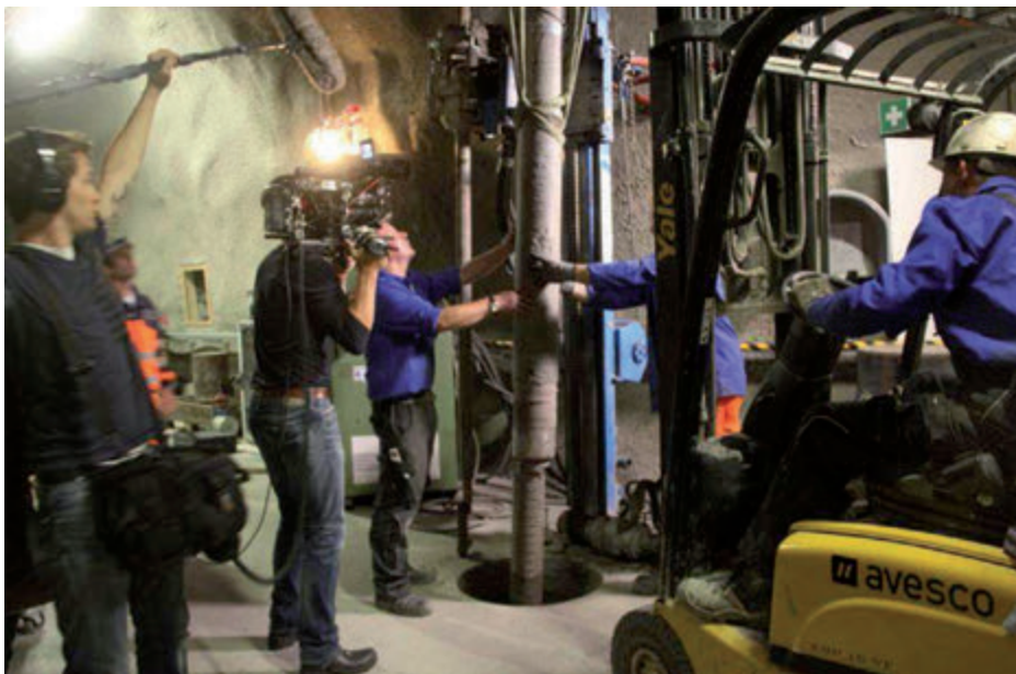
Figure 1. Overcoring of the CS experiment at Mont Terri rock laboratory.
