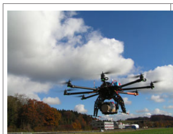
Figure 1: Octocopter with a radiation detector as payload.
