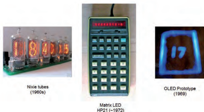
Fig. 1: Electronic displays end of 1960s: a) Nixie tubes, b) dot matrix LEDs, c) first OLED prototype of 1969 (~20x20x1mm).
