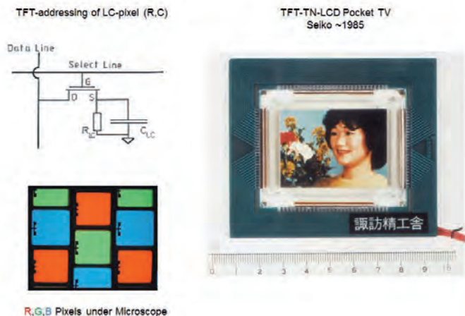
Fig.7: Thin-film transistor (TFT)-addressing scheme and microphotograph of the R, G, B color filters pixels of an early television TFT-TN-LCD.
