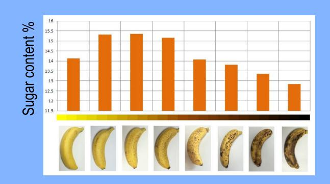
The sugar content is measured with a refractometer and a graph drawn showing sugar content versus ripeness.
