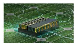
semiconducting nanowires, a technology usually employed for low-power applications, that has half as much resistance as conventional high-power transistors and can hold voltages of more than 1000 V. The key innovations of this technology are the use of a smart geometry for multiple nanowires in parallel, and the choice of gallium nitride, a semiconducting material ideal for power applications.
