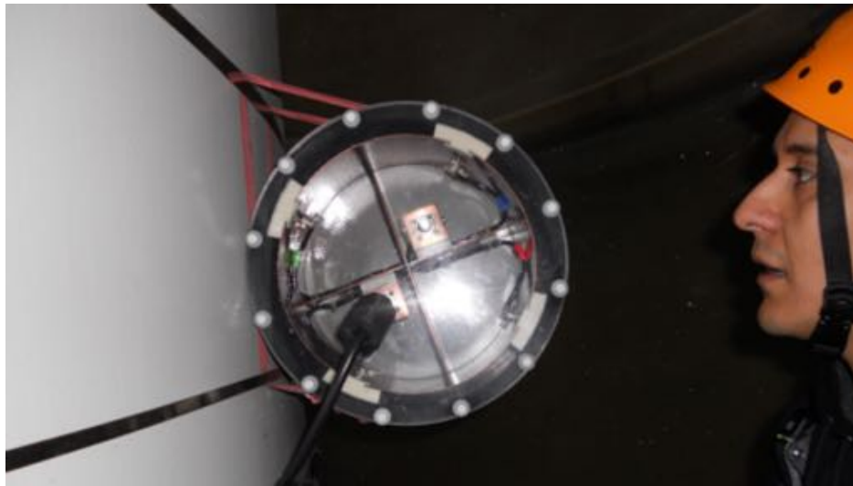
B-Dot installed along with Rogowski Coils
