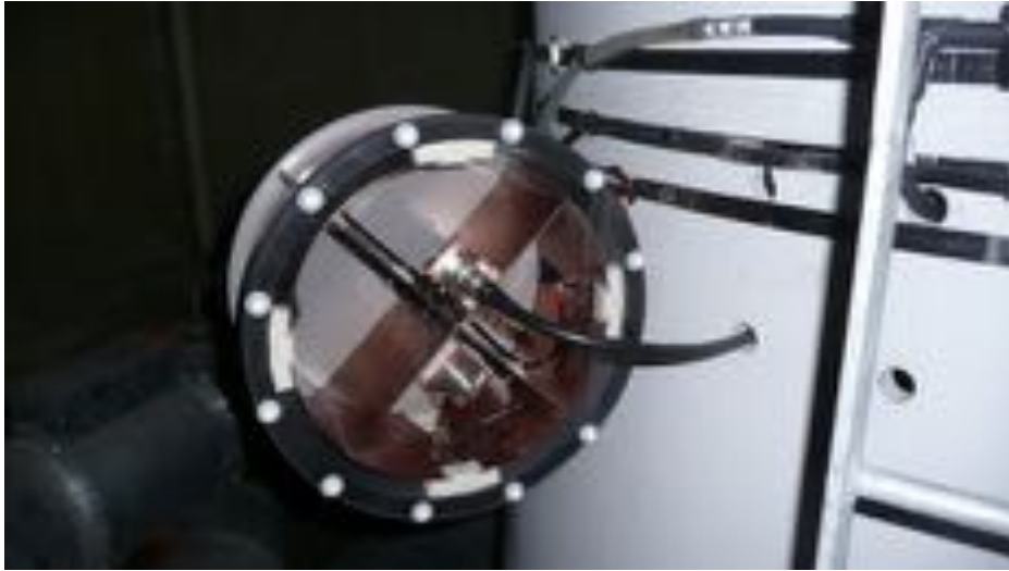
B-Dot installed along with Rogowski Coils
