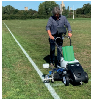
Figure 4: GNSS guided Line Marker © Fleet Line Markers Ltd.
