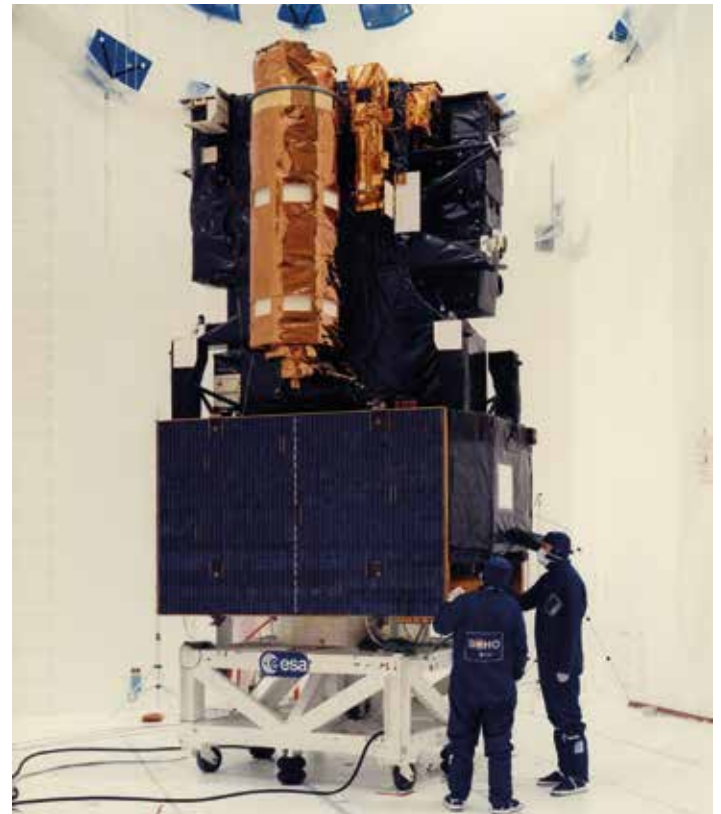
Figure 4: The SOHO spacecraft photographed during its laboratory tests. In its halo orbit, SOHO is three-axis stabilised and points continuously at the Sun.
