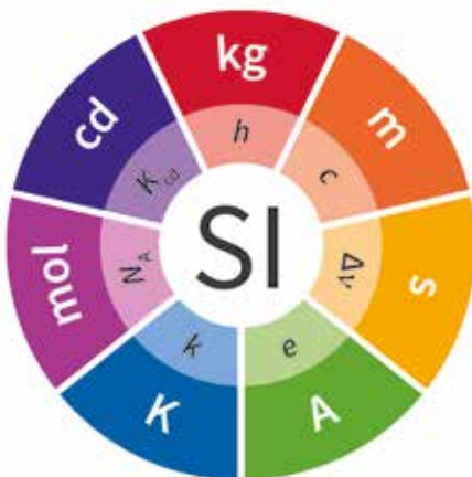
5: The revised SI: The inner circle shows the 7 defining constants. They form the building blocks for the realization of units shown on the external circle. The seven base units of the SI are shown. All other units can be derived from combinations of the defining constants. Base and derived units are equivalent.
