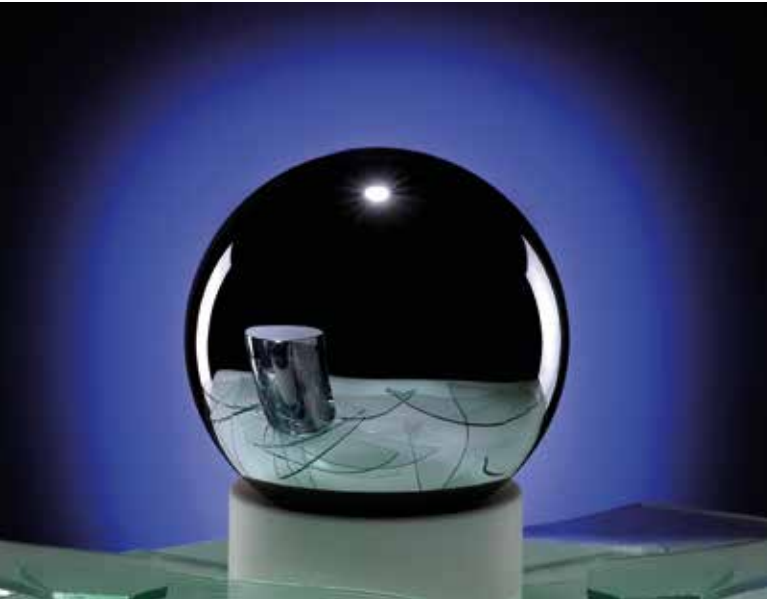
A silicon sphere helps to pave the way for the upcoming redefinition of the International System of Units (SI). Read the article on p. 26. (Picture: © Physikalisch-Technische Bundesanstalt Braunschweig)
