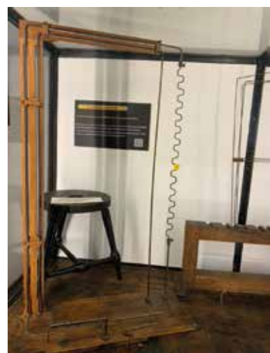
Figure 2: Experimental setup where an electric current flows through a conductor. The magnetic field lines were measured using magnetized needles at various distances to the non-uniform conductor. (Donation of the University of Geneva) (© HP Beck)
