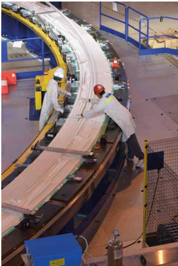
Winding and insulating a 24 m diameter PF coil at the ITER PF coils winding facility. © AP
