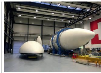
To run the new out-of-autoclave process for payload fairings, RUAG has invested in a state-of-the-art manufacturing hall in Emmen, Switzerland.
