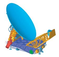
CAD model of the SWI telescope and receiver unit.
