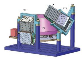
CAD model of the ICI on-ground calibration targets.
