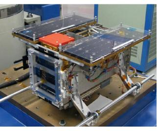
CLARA (with red cap) mounted on the NorSat-1 structure.
