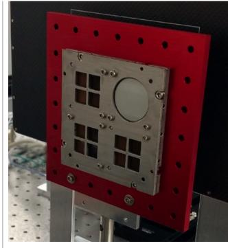
The MiSolFA Engineering Model is prepared for the first X-ray measurement of its Moiré inteference pattern.
