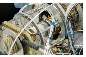
NIM prototype model for PEP/JUICE, mounted in calibration setup.
