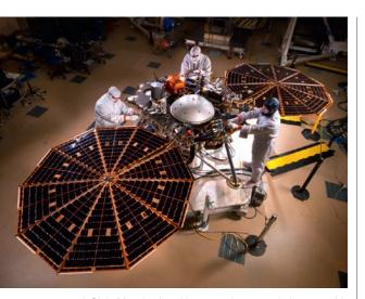
InSight Mars lander with open solar arrays during assembly and integration at Lockheed Martin.
