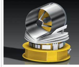
The SPICA satellite (Planck configuration, 2.5m@8K telescope).
