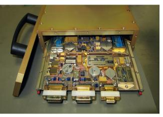
The FM of the Low Voltage Power Supply (LVPS) for the SPICE instrument built at PMOD/WRC and as delivered to ADS.
