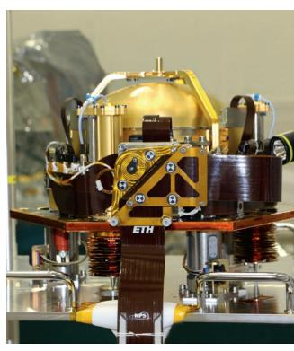
SEIS sensor assembly during integration at CNES.
