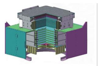
A sketch of the DAMPE payload showing the sub-detector systems.
