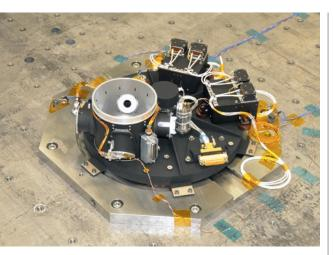
The Hitomi Filter Wheel Mechanism ready for the vibration test. Image credit: Ruag Space AG.
