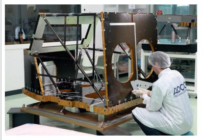
APCO Technologies is in charge of the Structure and Thermal Subsystem of the Sentinel 2 Multi Spectral Instrument of the Copernicus programme.
