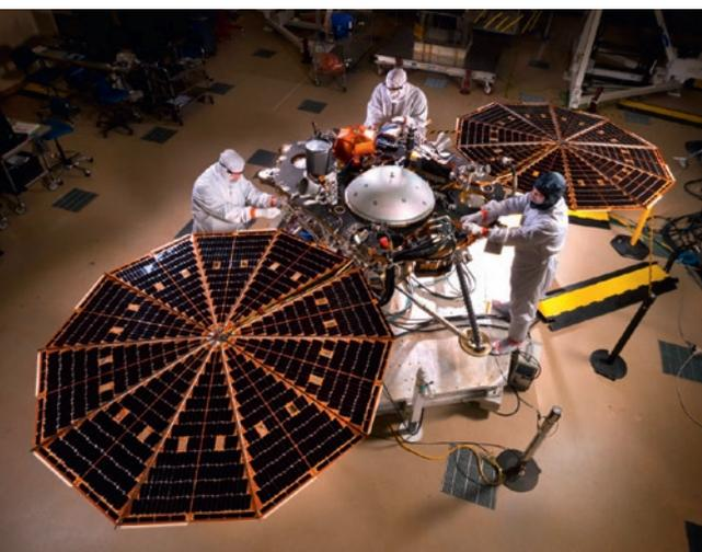
*InSight Mars lander with open solar arrays during assembly and integration at Lockheed Martin.*
