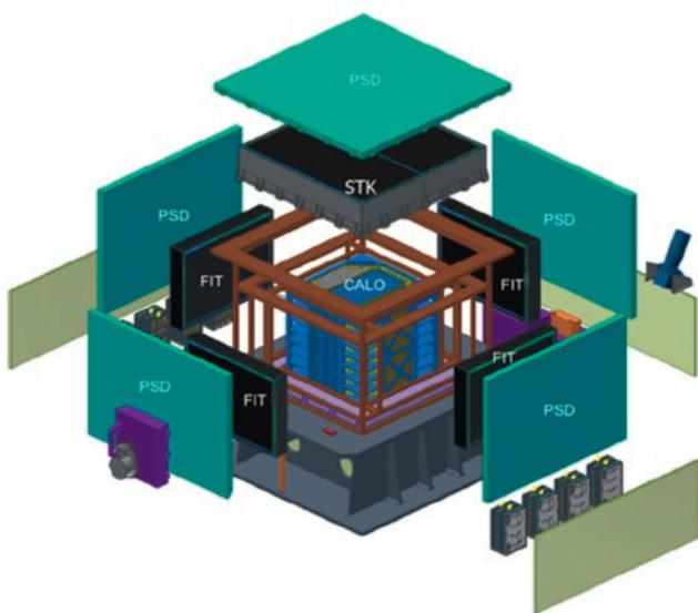
Sketch of the HERD detector: the 3-dimensional LYSO calorimeter (CALO) in the center, is surrounded by the 4-sided scintillating fibre tracker (FIT) and surmounted by the silicon-tungsten tracker (STK). The tracker is encapsulated in the 5-sided plastic scintillator detector (PSD).
