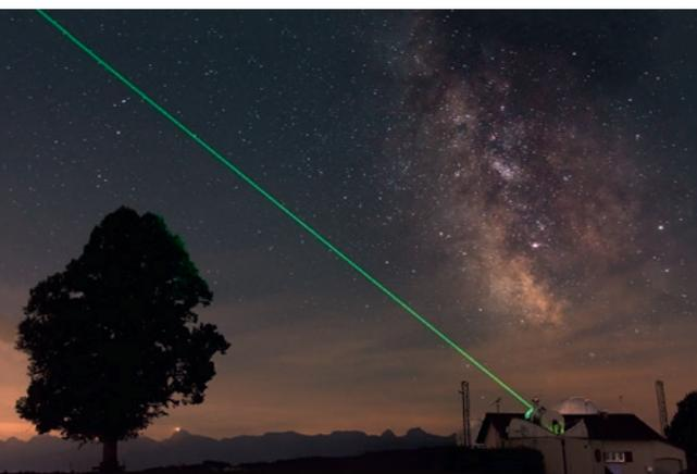
Laser beam transmitted from the 1-meter ZIMLAT telescope to measure high accuracy distances of artificial satellites.
