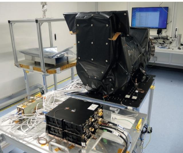
The CHEOPS electronics boxes. On the right is the BEE (Back End Electronics) housing the Data Processing Unit (DPU) and the power converter. On the left, the SEM (Sensor Electronics Module) which controls the CCD as well as the temperature stabilisation of the focal plane module. Both boxes will be housed in the body of the spacecraft.
