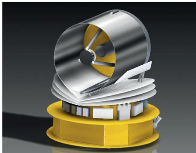
The SPICA satellite (Planck configuration, 2.5m@8K telescope).
