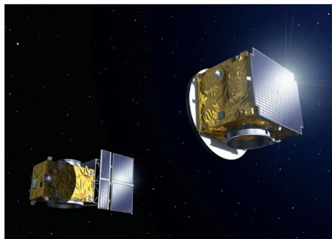
PROBA-3 is an ESA formation-flying technology demonstration. Two satellites will fly with a 150 m separation on a highly elliptical orbit (600 x 60530 km). DARA is mounted on the front platform. Image credit: ESA.
