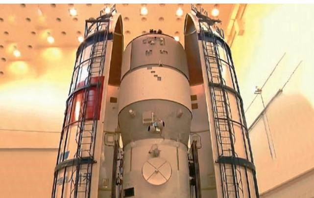
POLAR can be seen integrated on Tiangong-2 which is attached to the "Long March" rocket just before the fairing is definitely closed.
