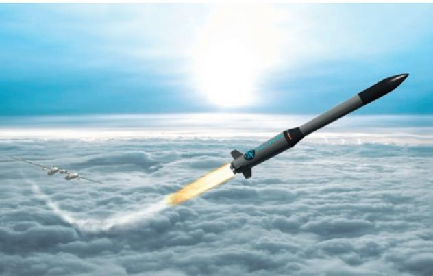
The ALTAIR carrier and launcher performing the separation manoeuvre.
