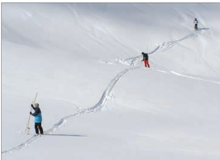
Photo 5: Performing BTS measurements at Alpage de Mille; GPS survey permits to locate BTS points every year at the same places (precision : \pm 5 m). Photo: R. Delaloye, March 2004.
