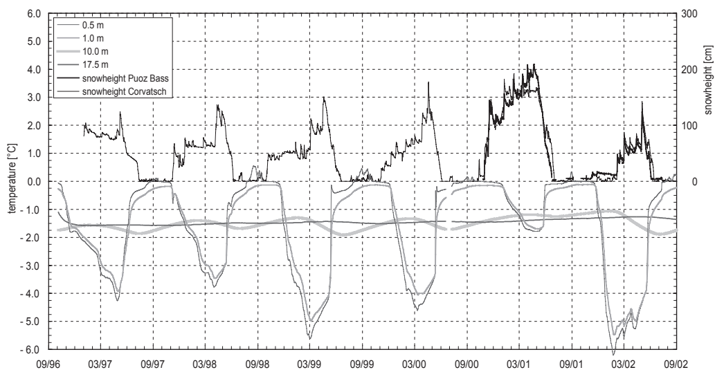
Fig. A.23: Temperature-time plot of the borehole Schafberg-Pontresina 2/90 for the thermistors at 0.5, 1.0, 10.0 and 17.5 m depth. Additionally, the snow height at Puoz Bass and on Corvatsch is displayed.
