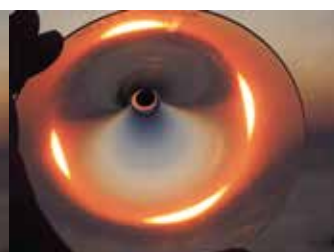
An optical lens with the shape of a wine glass bottom simulates the gravitational strong lensing effect: a classroom experiment to reproduce Einstein's rings, crosses and arcs (from the talk by Alice Gasparini). The session report is on p. 13.
