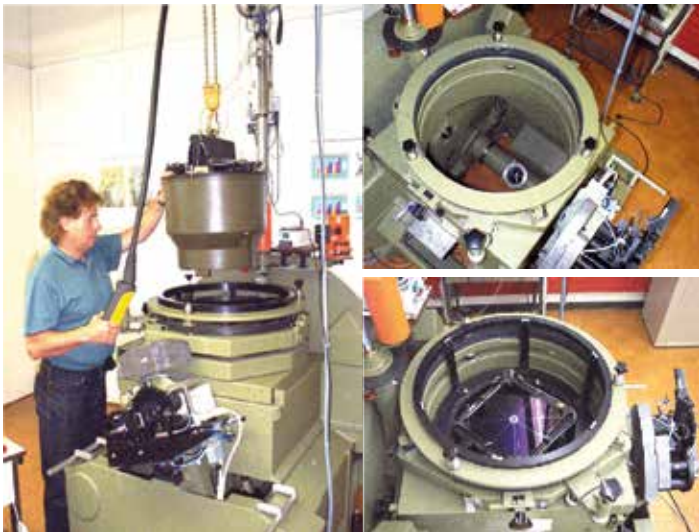
Fig. 1: Calibration of a film lens Universal Aviogon UAGS-2 with the electronic vertical goniometer EVG.
