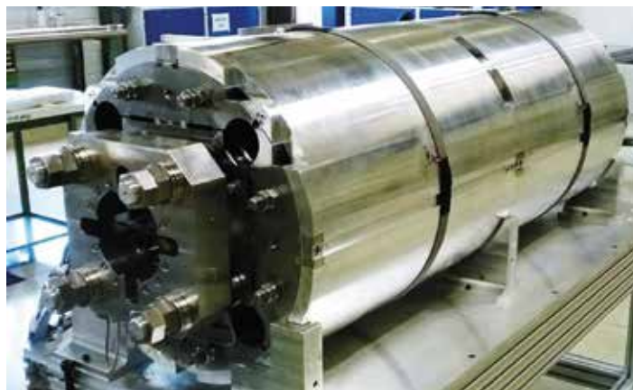
Figure 3: A forged and rolled Aluminium magnet body at Imbach AG (prepared for the CERN High Luminosity LHC project). © CERN
