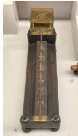
Fig. 10: One of the first horseshoe magnets ever made, carrying more than 30 kg, made by the goldsmith Johann Dietrich in 1755, who built several instruments for the Cabinet (photo Maurice Babey, Basel).
