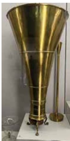
Fig. 8: "Hydrostatic Paradoxon" Device for demonstrating the Hydrostatic Paradox, with the following description: A wide and a narrow vessel are screwed on the same cylinder. If the water column is the same, the bottom pressure in both vessels is the same. This hydrostatic paradox states that the gravitational pressure exerted by a liquid in a vessel on the bottom of the vessel, while dependent on the level of the liquid, is, on the other hand, independent of the shape of the vessel and thus of the quantity of liquid contained - an example of the fundamental insights of Daniel Bernoulli. Manufacturer: Johann Ulrich Goetz (1694 - 1758), Basel, 1728, since 1757 in the collection of the Institute of Physics of the Univ. of Basel (photo Salome Noah, Basel).
