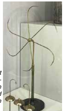
Fig. 9: Musschenbroek's pyrometer (thermal expansion meter), as an example for Bernoulli's lectures with experiment demonstrations: The device was used to demonstrate the expansion of metal under heat. In this process, an iron rod is heated by six spiritus flames and its expansion or coefficient of expansion is indicated by a special transmission mechanism with a pointer on a dial. The pyrometer of this type was invented in 1731 by the Dutchman Pieter van Musschenbroek (1692 - 1761). Made by Jean Pierre Charme, Paris, ca. 1752, iron, brass, wood; purchased by Prof. Daniel Bernoulli (photo Salome Noah, Basel).
