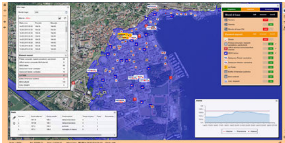
Figure 1. SITGAP 2.0 Web interface illustrating a simulated active alarm with lake level forecasts, inundation area and exposed elements.
